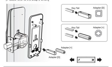
\* When using the Adapter D, insert the "L" direction into the key tail side if the door opens to the left, otherwise insert the "R" direction into the key tail side if the door opens to the right. [If it is reversed, the door lock will not work properly.]
