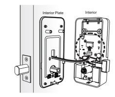
7 Make sure that the cable is not caught, and place the Interior Plate and the Interior Unit to the Thumb-Turn and the Adaptor direction. When attaching the Adapter, make sure it is horizontal, and check if the deadbolt moves smoothly by rotating the Thumb-Turn.
